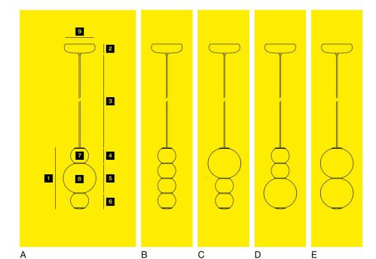
340 mm 50 mm Max. 2500 mm Height Adjustable 80 mm 165 mm 80 mm Ø100 mm 8 Ø180 mm Ø170 mm
